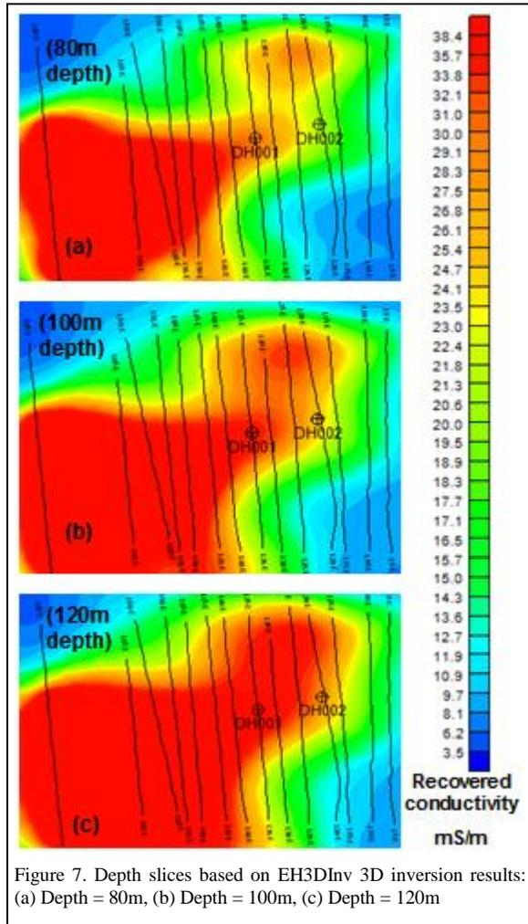
Figure 7. Depth slices based on EH3DInv 3D inversion results:
