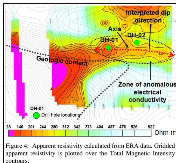
The zone of anomalous electrical conductivity shown in Figure 3 appears to be a down-dip continuation of the ultramafic pluton, which is at the same time consistent with the rapid change in Total Magnetic Intensity, marking the geologic contact. Based on this interpretation two drill holes (DH01 and DH02) were planned. DH01 appears to be consistent with the axis of the anomalous zone, while DH02 is located down-dip from the axis.
