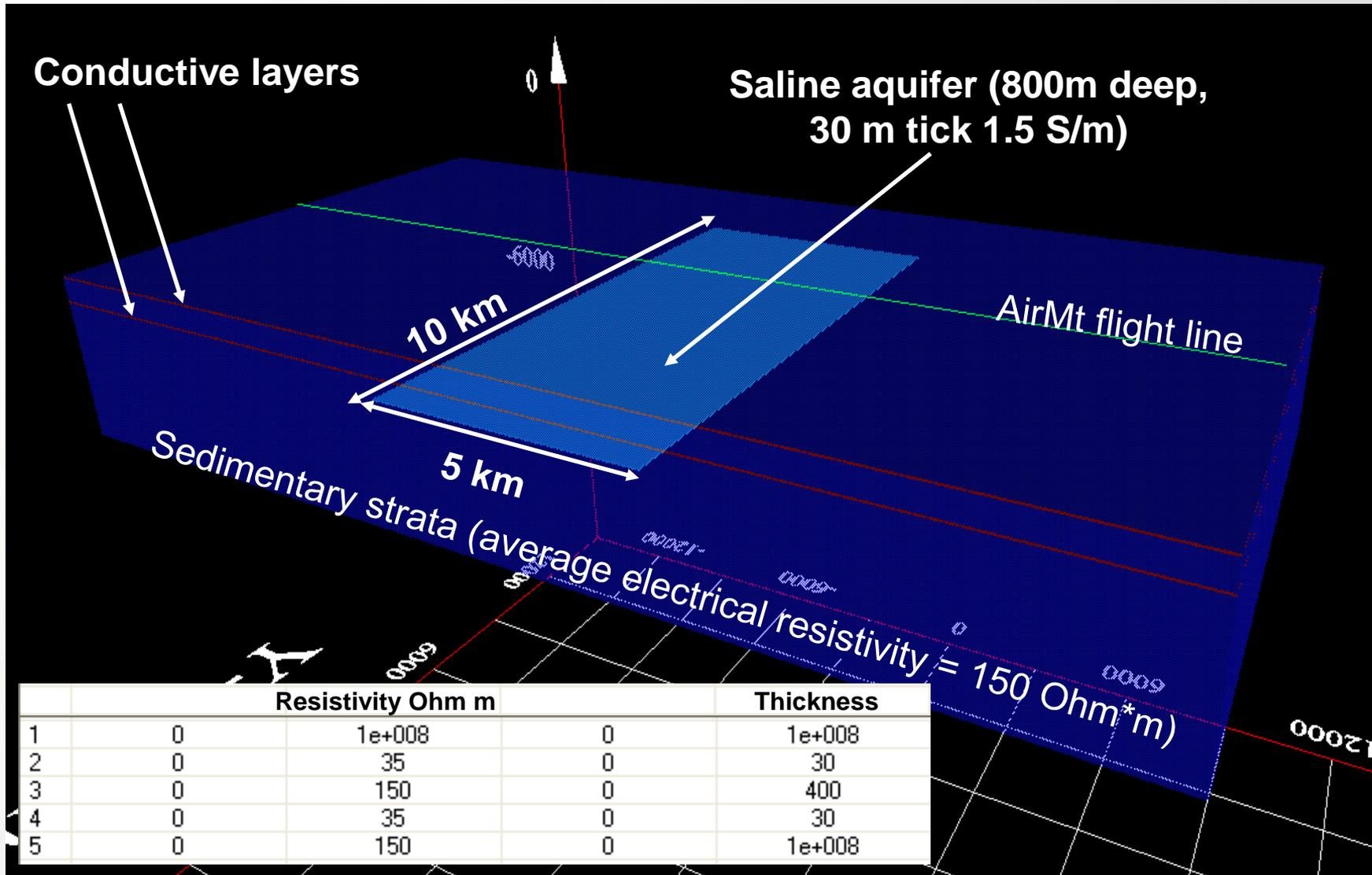
Saline aquifer electrical resistivity was initially set at 1.5 S/m and gradually decreased simulating the sequestration process
