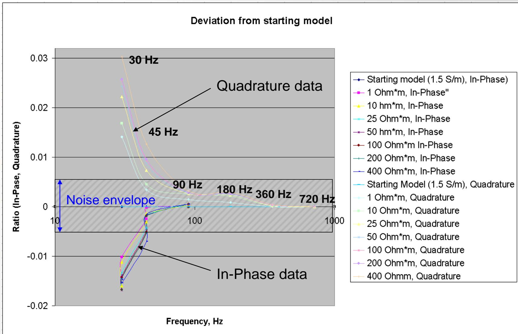
These curves were acquired from modeling of 800m deep saline aquifer at different stages of sequestration process
